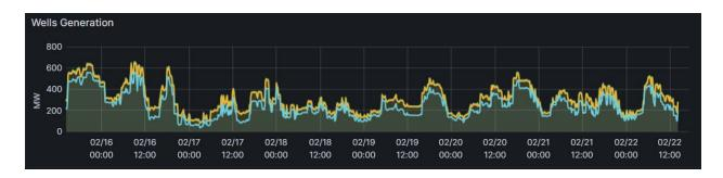
The data demonstrate two things: 1) Wells Dam rarely operates at or near its nameplate capacity, and 2) the ability of hydropower to follow load by increasing and decreasing generation instantaneously.
