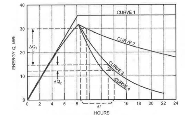
Fig. 17 Typical Storage Heater Performance Characteristics (Hersh et al. 1982)
