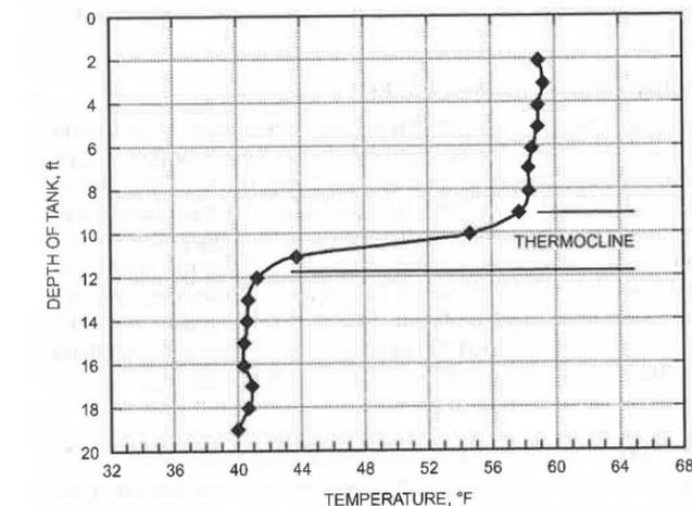
Fig. 2 Typical Temperature Stratification Profile in Storage Tank
