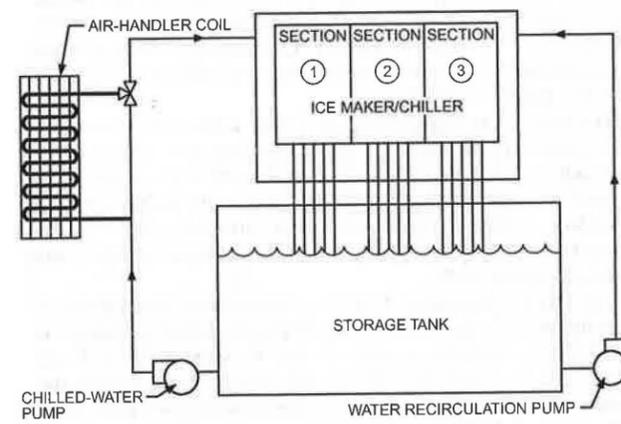
Fig. 15 Ice-Harvesting Schematic
