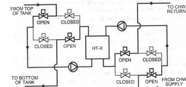
Fig. 29 Charge Mode Status of Indirect Transfer Pumping Interface
