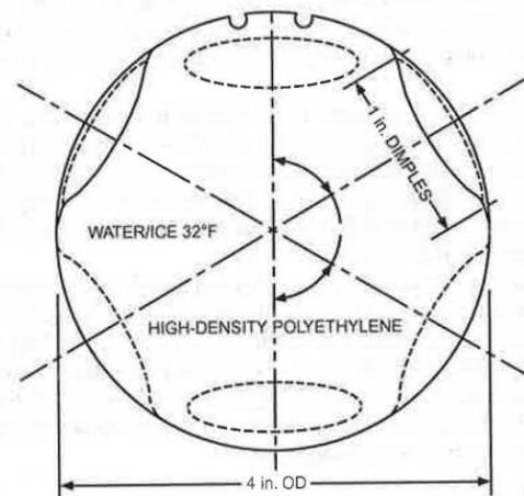
Fig. 14 Encapsulated Ice: Spherical Container
