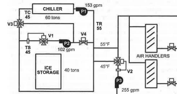
Fig. 33 Parallel Flow for Chiller and Storage
