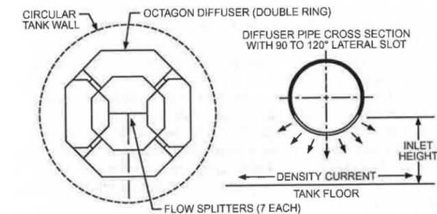
Fig. 1 Typical Two-Ring Octagonal Slotted Pipe Diffuser
