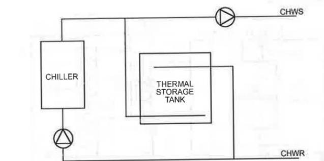
Fig. 30 Primary/Secondary Chilled-Water Plant with Stratified Storage Tank as Decoupler
