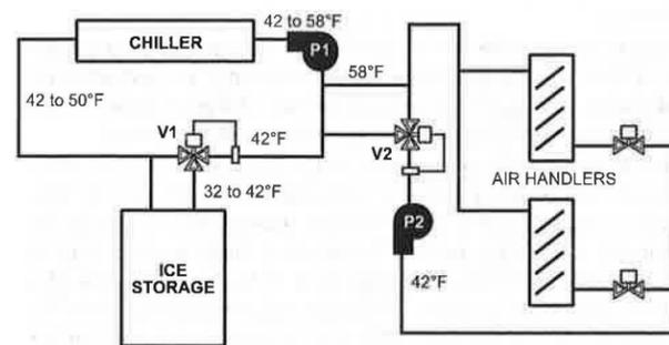
Fig. 31 Series Flow, Chiller Upstream
