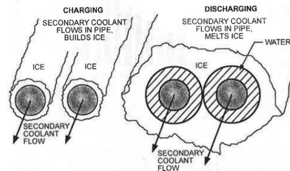
Fig. 9 Charge and Discharge of Internal-Melt Ice Storage
