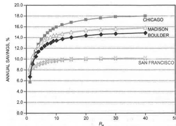
Fig. 23 Annual Energy Cost Savings from Precooling, Relative to Conventional Controls, as Function of  $R_e$
