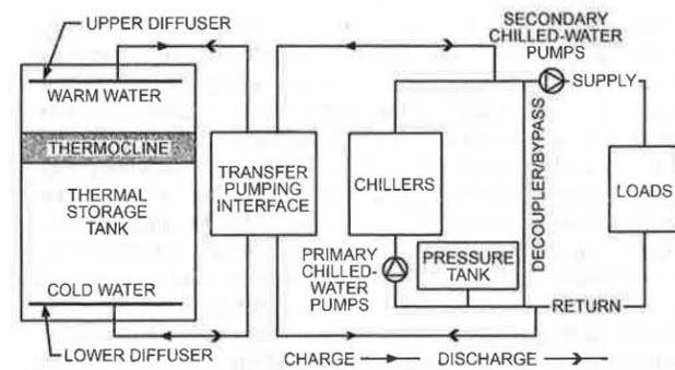
Fig. 25 Typical Sensible Storage Connection Scheme
