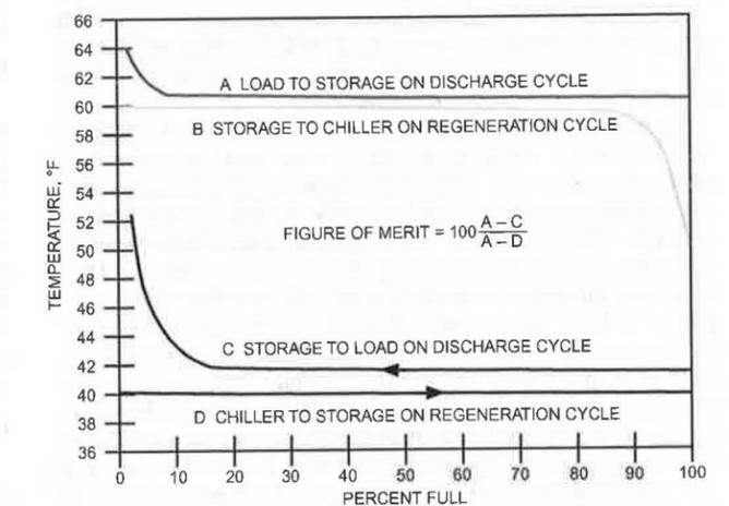
Fig. 3 Typical Chilled-Water Storage Profiles
