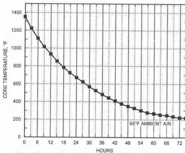
Fig. 20 Static Discharge from Room Storage Heater
