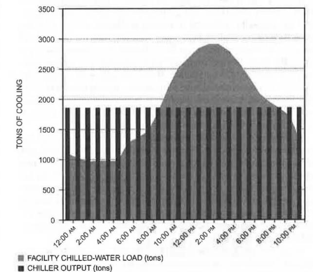
Fig. 7 Cooling Load (tons) and Chiller Load (tons) with Partial-Storage TES Tank
