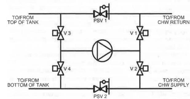
Fig. 26 Direct Transfer Pumping Interface
