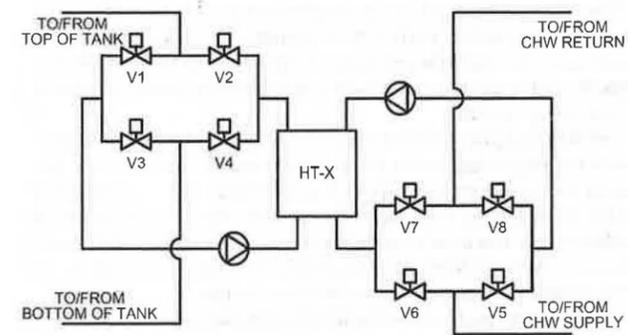
Fig. 28 Indirect Transfer Pumping Interface
