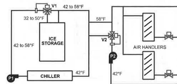
Fig. 32 Series Flow, Chiller Downstream
