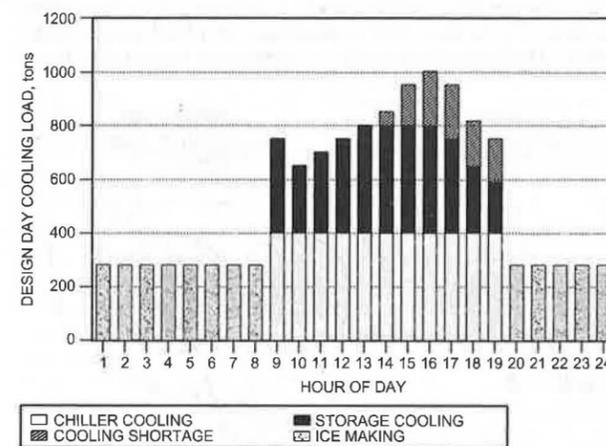
**Fig. 12 Redundancy with One of Two Chillers Disabled**
