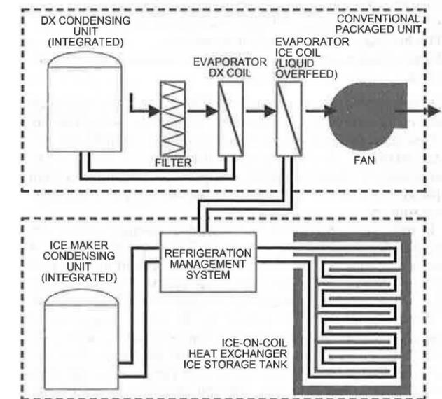
Fig. 34 Typical UTSS with Packaged DX Equipment (Willis and Parsonnet 2010)
