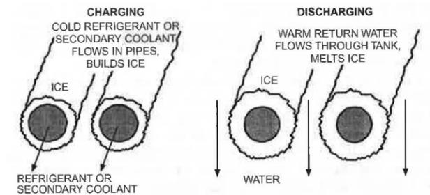
**Fig. 13 Charge and Discharge of External-Melt Ice Storage**
