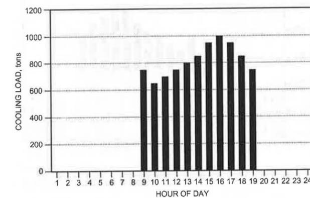
Fig. 10 Design-Day Cooling Load
