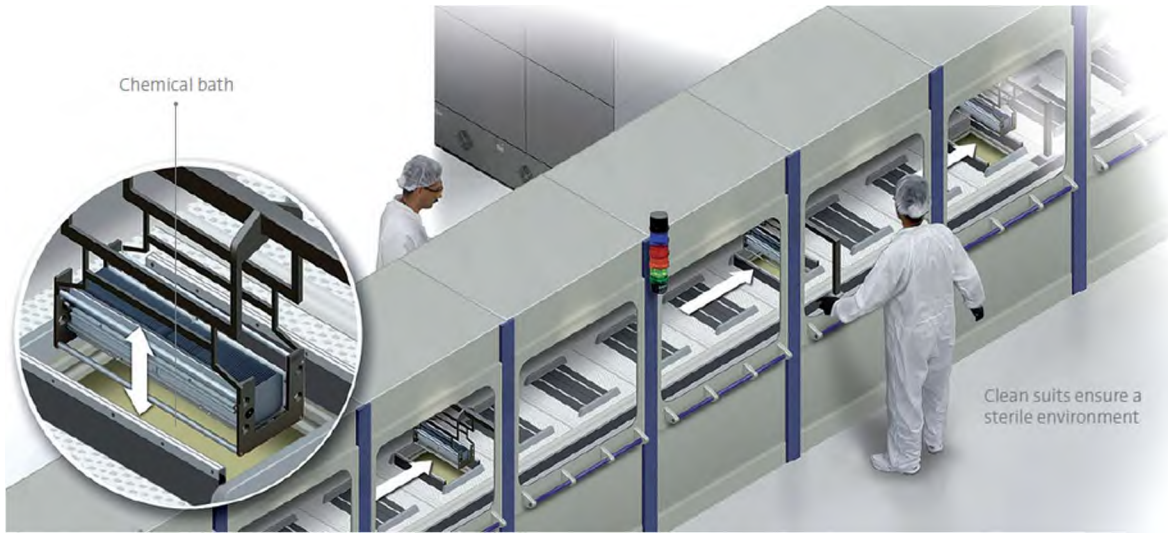
Figure I-16 CSPV cell production: Texturing (top) and screen printing (bottom)
