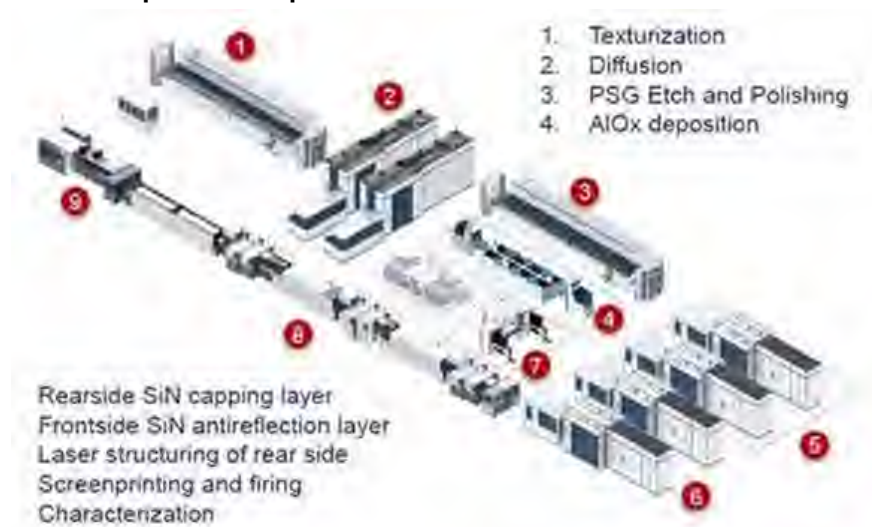
Figure I-17 CSPV cell production process
