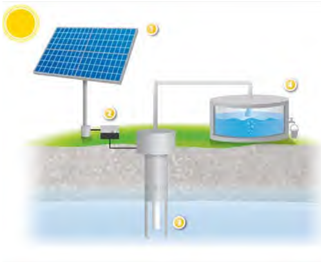
Figure I-6 Off-grid water pumping system (left) and light system (right)
