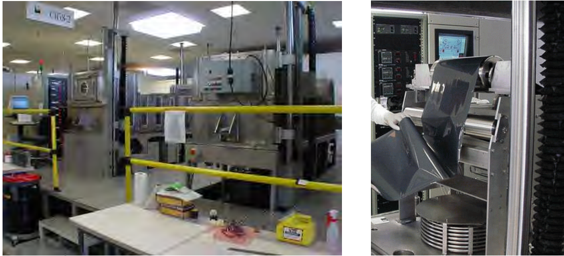
Figure I-10 Roll to roll CIGS production equipment (left) and CIGS on a flexible substrate (right)
