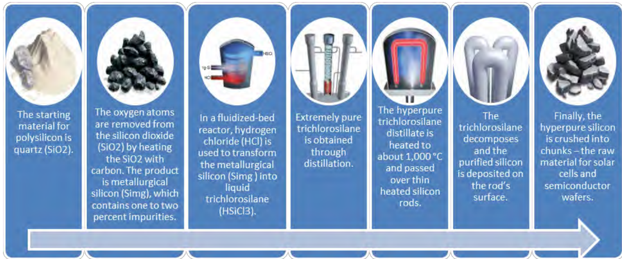
Figure I-13 CSPV products: Polysilicon refining process (Siemens method)
